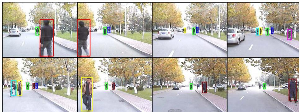
Fig. 11. Tracking examples in the SDL-Campus data set from the frame 1290 to 1413, which includes many pedestrians more than 25 meters away from the moving platform, their observation regions are smaller than those in the above data sets. The results come from the proposed LGM method.
