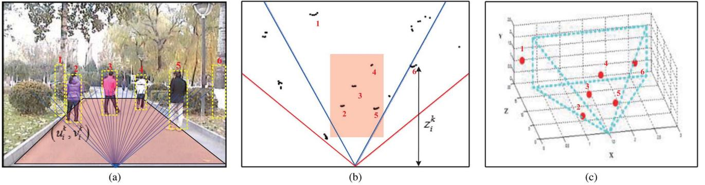
Fig. 2. (a) Pedestrian observations in the RGB domain and (b) observations in the D domain. The red and blue lines denote the scanning range from the D and RGB sensors, respectively, (c) observations are projected to 3-D space which combines the RGB and D data.
