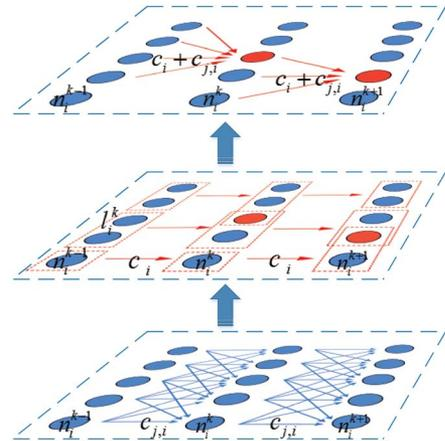
Fig. 3. The layered graph model. A fully-connected graph is in the bottom part, where all the nodes in the adjacent frames are connected, and  $C_{j,i}$  is the edge cost. In the middle part, the nodes are divided into different layer marked with red dashed rectangles. The edges connecting the nodes exist inside of the layer. The red nodes in the overlap regions belong to adjacent layers. In the upper part, the edges connecting the nodes of overlap regions exist in the adjacent frames.
